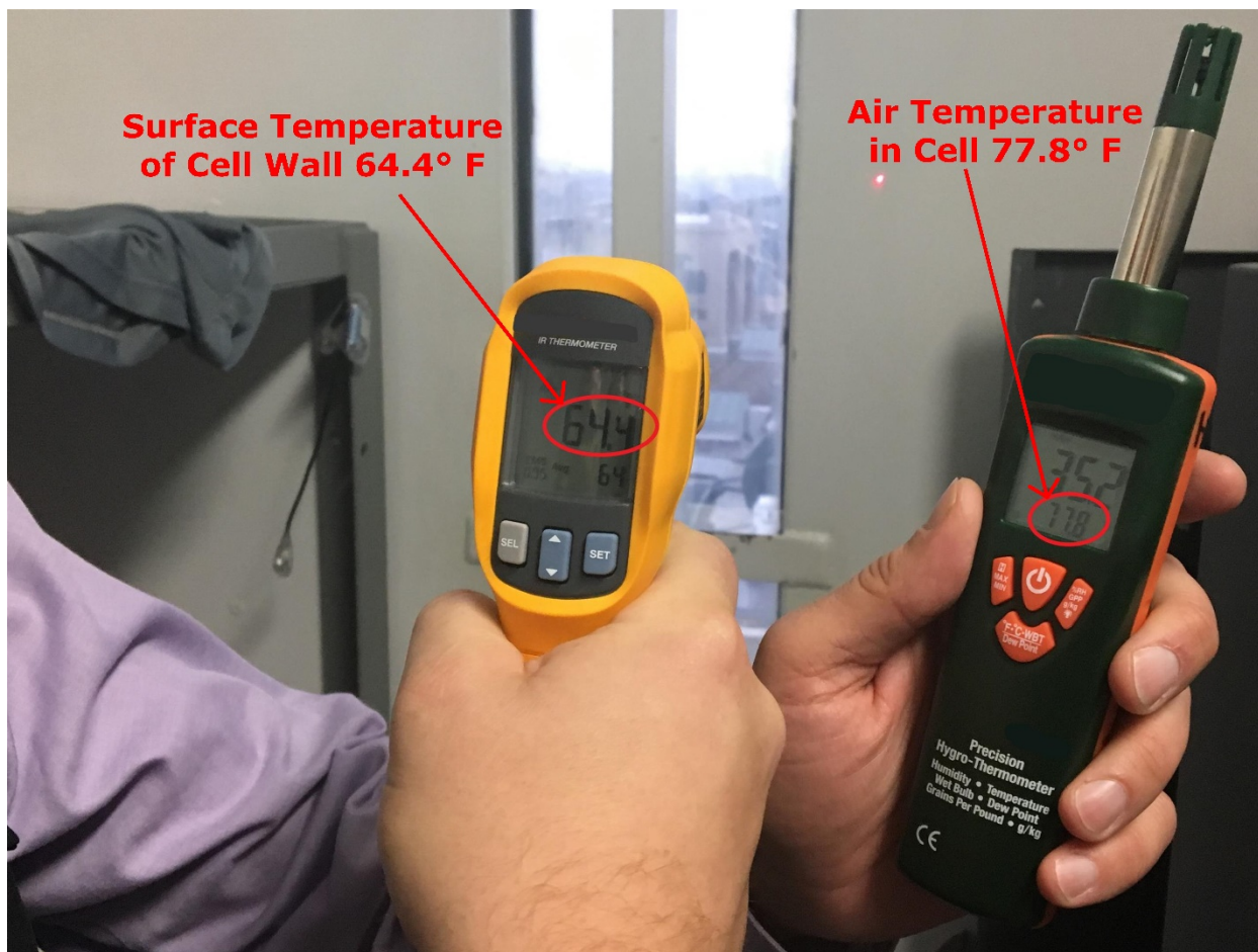
Photograph 3: Exterior Wall Surface and Ambient Air Temperature Differences in an Inmate Cell
