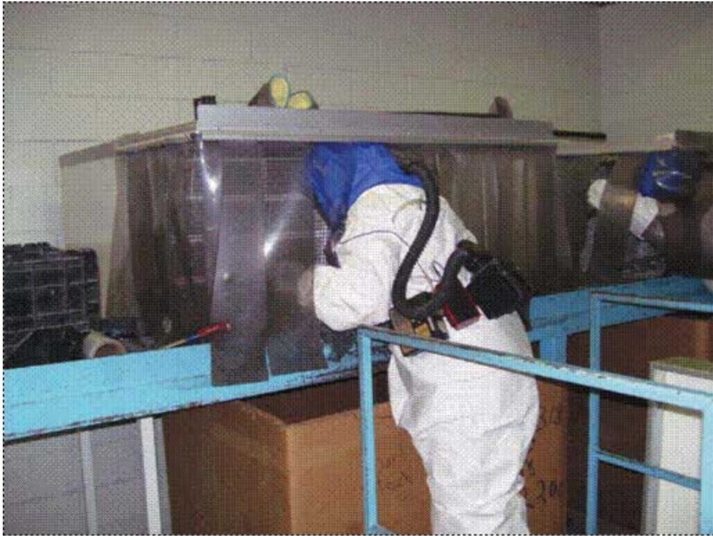
Image 1: Glass breaking operation by workers in PAPRs and disposable coveralls
