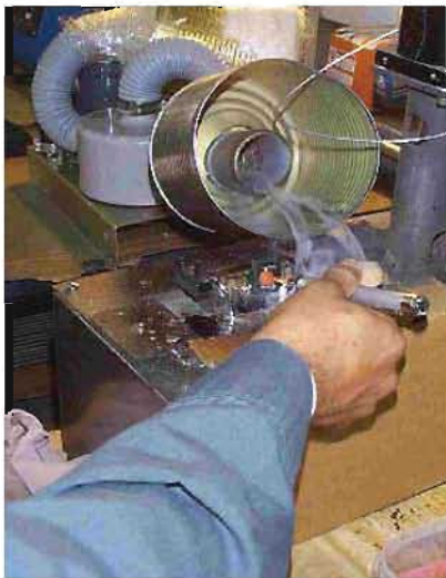
Images 3 and 4. Chip recovery stations showing use of LEV and PPE
