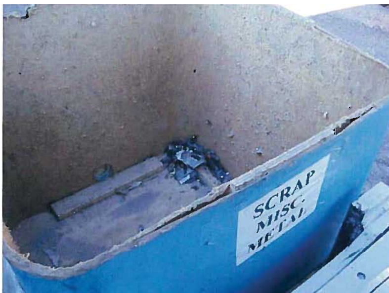
Image 4. Debris in scrap metal roll-off container (similar to debris constituting the sample exhibiting TCLP lead levels above RCRA hazardous waste limit).
