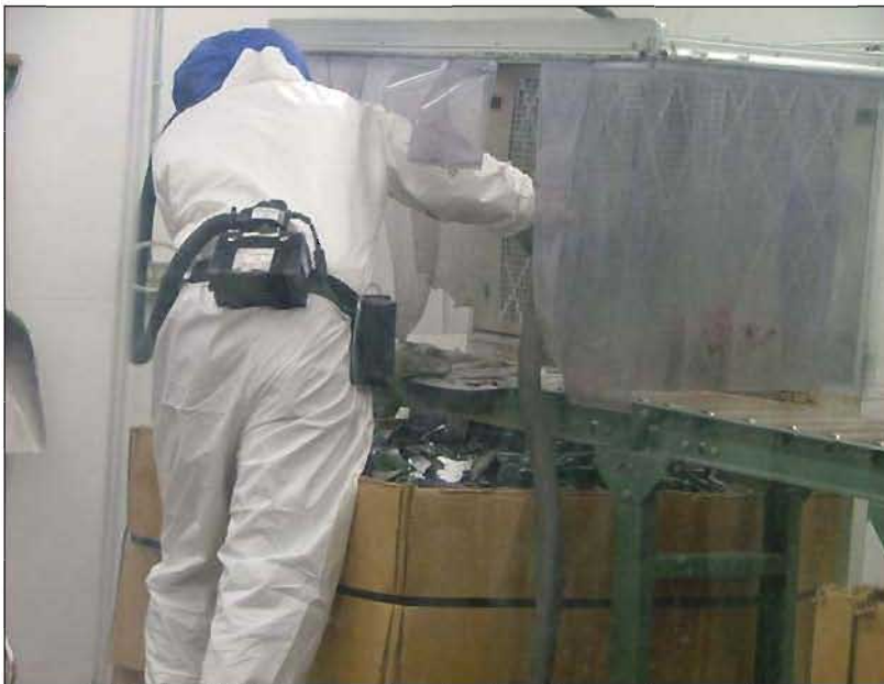
Image 2. Worker HEPA vacuuming glass breaking station wearing a powered air purifying respirator (PAPR)
