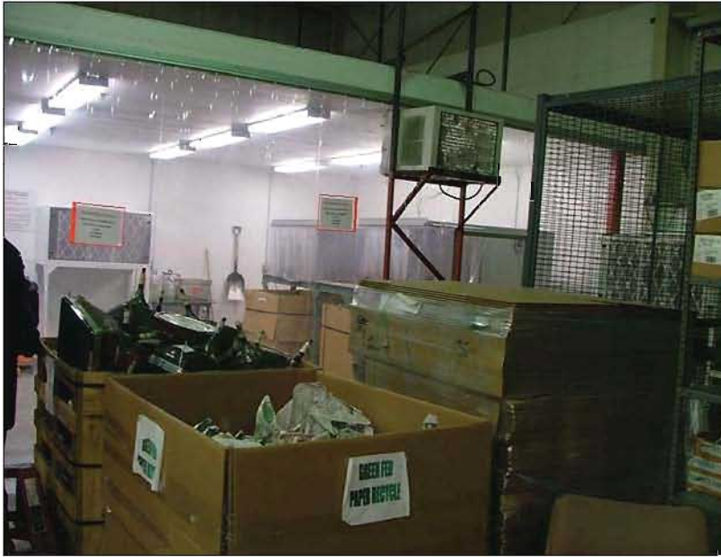
Image 1. Glass breaking room (in background) with containers of CRTs outside the glass breaking enclosure awaiting breakage
