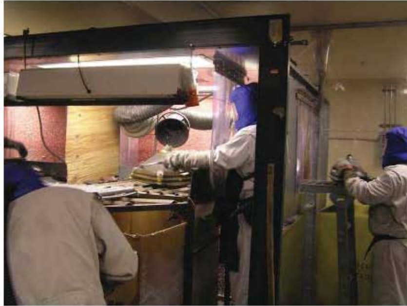
Figure VII Electron Gun Removal in Glass Breaking Operation
